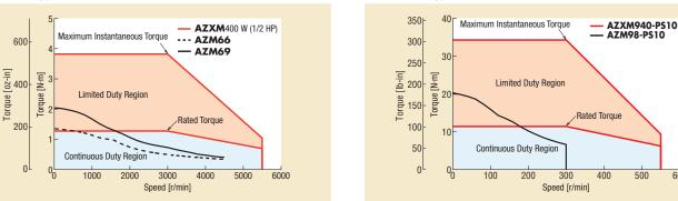
This is a comparison of the speed – torque characteristics of the AZX Series and AZ Series.
