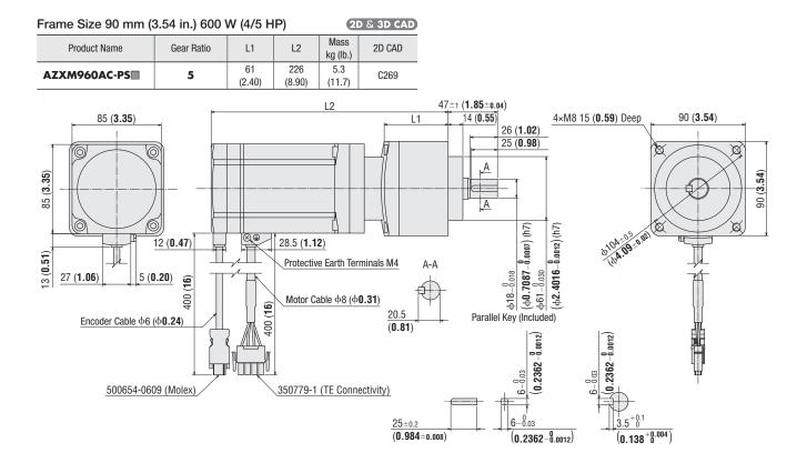
A number indicating the gear ratio is specified where the box is located in the product name.
