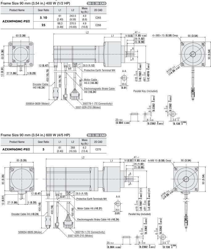
A number indicating the gear ratio is specified where the box is located in the product name.
